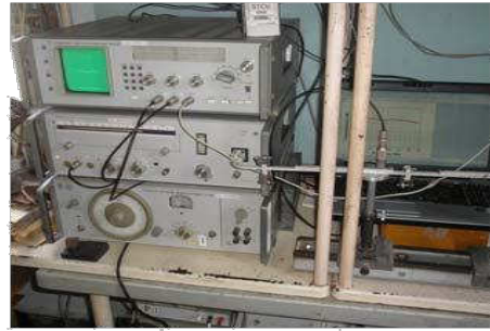
Fig. 5.10. The experimental setup for the frequency range of 26 – 37.5 GHz.
